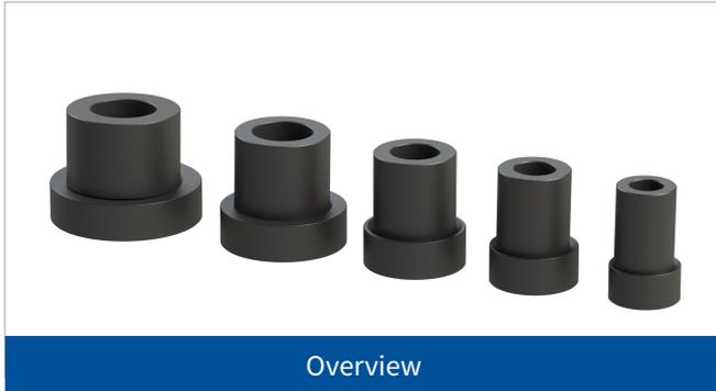
The MecLev® Spherical Extension Sleeves (SES) is a bush combined with a spherical washer on one end, that assures 100% nut pull on critical bolt and stud assemblies. The SES elements are designed in order to combine the functionality of creating extra stretch length to bolted connections, as well as correcting angular misalignment between bolted planes up to 4°.
